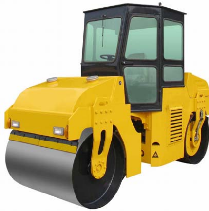
Tandem Vibratory Roller(Mechanical Transmission) LGC206
